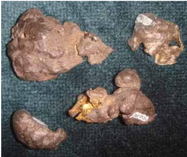
Fig. 3. The largest piece of silver alloy contains 20% of copper and only traces of gold (Inv. No. 2002.21.75). This was most probably the original composition of the silver objects. This alloy could be used for vessels, boxes and mirrors.
