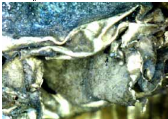
Fig. 2. Photo taken through the microscope showing the remains of a semi-molten gold sheet (Inv. No. 2002-21.74) in a silver lump.
